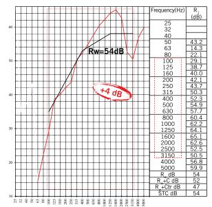
Trial report: TDC-09-ACOU-012-Rw of 18.03.2009: for a partition wall type D125/75/60, made of 2 NIDA Acustic 12,5 mm plasterboards on each face of the metal structure, consisting of CW75 profiles at an interaxis distance of 600mm, lined with a 50-mm thick fiberglass layer, the resulting acoustic insulation is Rw=54 dB\* + 4 dB compared to a standard system D125/75 (Rw= 50dB)
